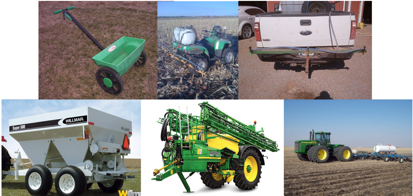
Figure 2. Equipment used for N-Rich Strips. From top-left to bottom right: Push spreader, ATV with 10-foot spray boom, receiver hitch mount with trigger in cab, dry fertilizer spreader, sprayer pull or self-propelled (often only use middle section) and anhydrous applicator.
