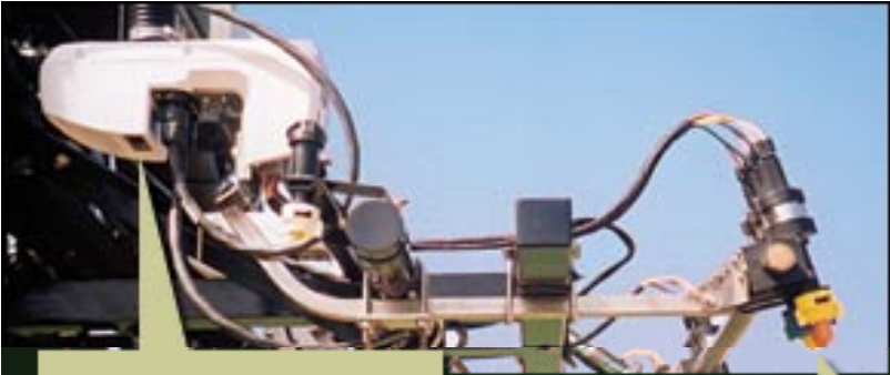
Spray nozzles apply fertilizer in a previously sensed area
